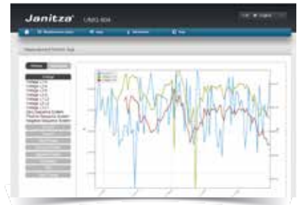
Fig.: Illustration of the online data via the device's own homepage
